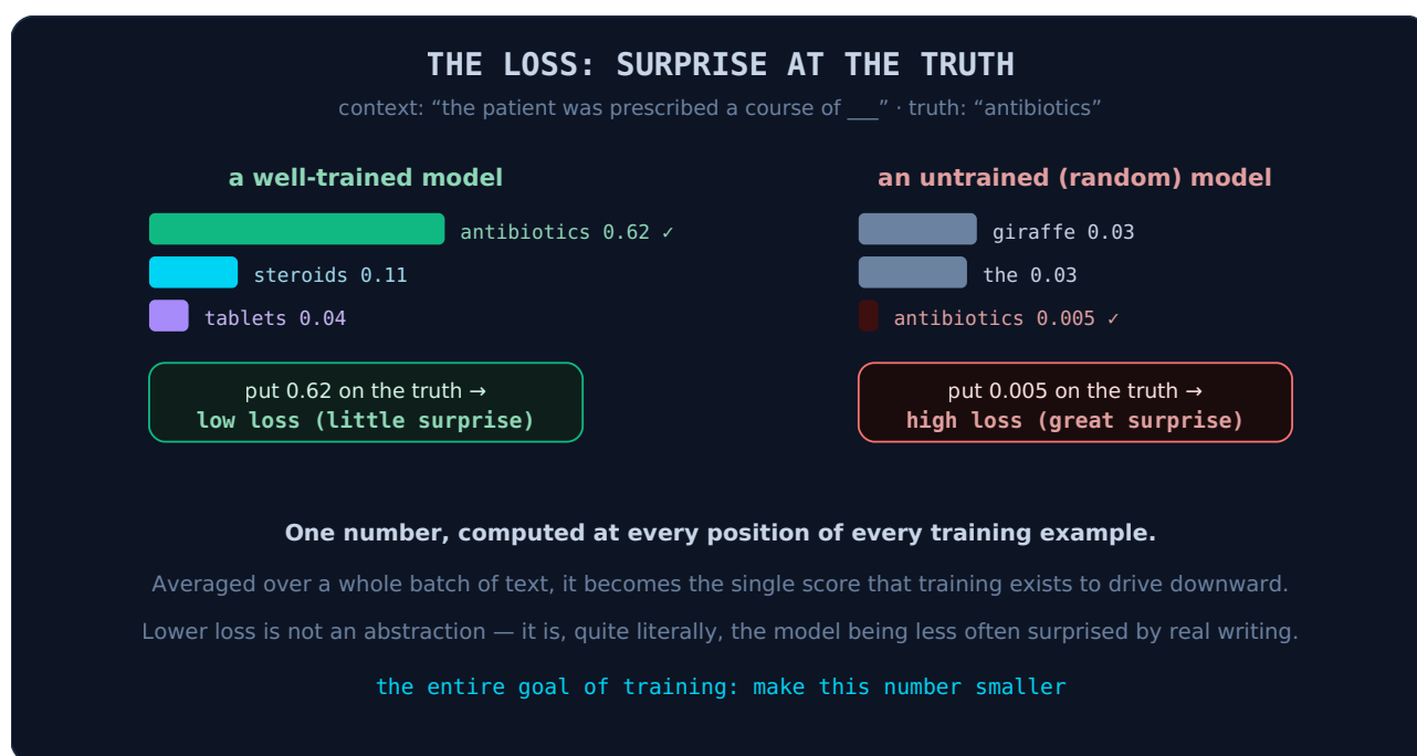
Figure 1. The loss turns "how wrong is the model right now?" into one number, by asking how much probability it placed on the token that actually came next. It is high for a confidently-wrong model and low for a confidently-right one. This single number — averaged over many predictions — is the compass for everything that follows.
