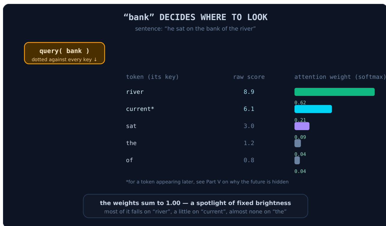
Figure 2. The scoring step for a single token. Its query is dotted against every key to produce raw scores; softmax turns those into attention weights that sum to one. Crucially, these weights are not stored anywhere — they are recomputed from scratch, from the actual content of this particular sentence, every single time. Change one word and the whole spotlight redraws.
