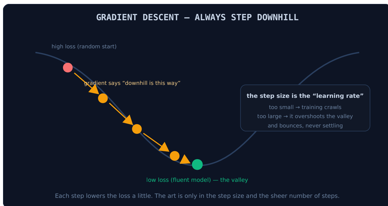
Figure 2. Gradient descent, the engine of all learning here. The loss is a landscape over the space of all parameters; the gradient reveals the downhill direction; we take a small step that way and repeat. The size of each step is the learning rate — one of the few dials a human sets — and getting it wrong in either direction (crawling, or overshooting and bouncing) is one of the most common ways training fails.
